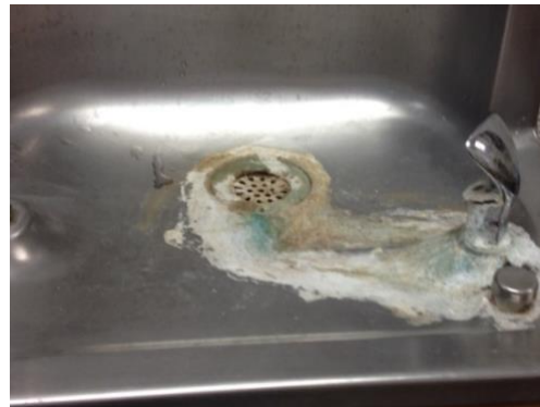
Figure C.1. Mineral deposits are calcium carbonate, indicating the drinking water is rich in minerals.
