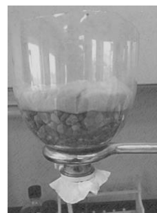
Figure 7.2. Coffee filter, pebbles, and sand filtration.
